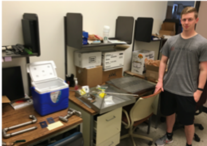
Methanol/Carbon Based Absorption Refrigerator/Ice Maker
