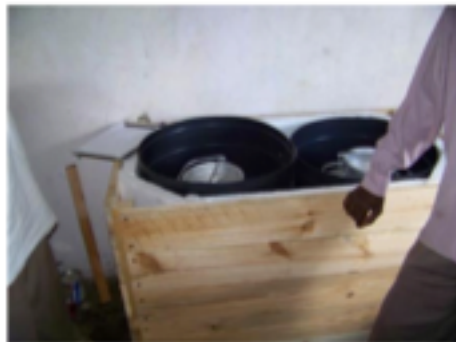
Figure 6. Milk is chilled in an ice-bath milk chiller. Each ISAAC produces enough ice to chill 100 liters per day.
