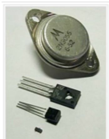
Assorted discrete transistors. Packages in order from top to bottom: TO-3, TO-18, TO-18, SOT-23
