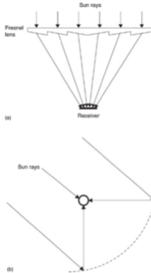
FIGURE 3.17 Fresnel collectors. (a) Fresnel lens collector (FLC). (b) Linear Fresnel-type parabolic trough collector.
