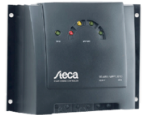
Figure 5.9 This MPPT controller can control a 12 or 24V system with PV array power up to 500W, and MPP voltages up to 100V. With dimensions 19 x 15 x 7 cm, it weighs 900g (Steca Elektronik GmbH).
