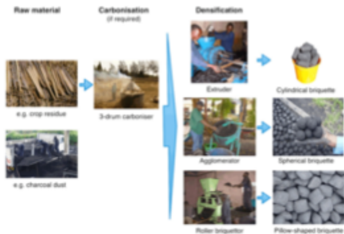
Fig. 2. Schematic diagram of "carbonize-first" briquetting method, in which raw biomass is carbonized (or salvaged in carbonized form) before it undergoes the densification process to form uniformly shaped briquettes.
